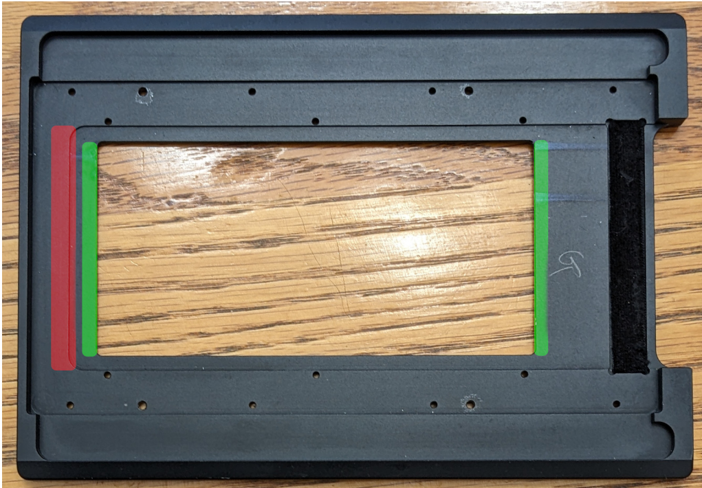
Graflok plate. Machine green areas all the way through and red area to the darkslide chamber height.
